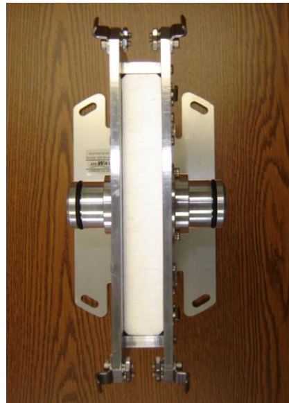
Four slots at antenna attachment points allow \pm 3^\circ polarization adjustment.
